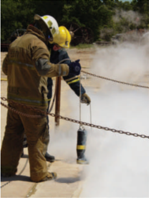
In this demonstration of embrittlement, a fireman's boot with steel toe cap is taken from an LNG pit. Pictures courtesy Resource Protection International
