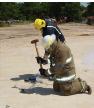
Using the same hammer, without much force, the pipe easily breaks up due to embrittlement.
