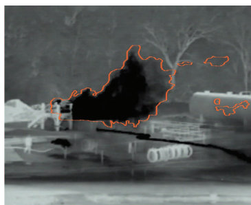
Vapour cloud before foam application. Picture courtesy Flameout.
