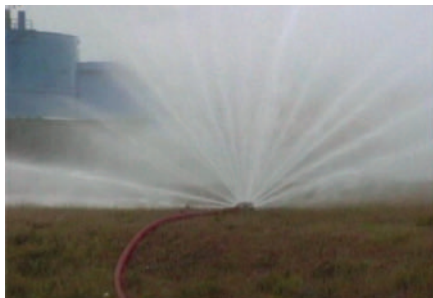
An example of a portable water curtain nozzle (Picture courtesy Resource Protection International.)
