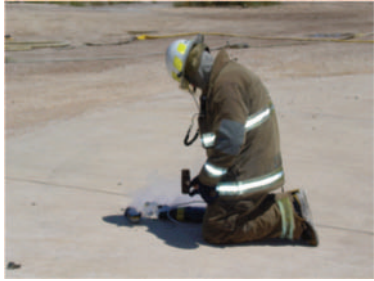
Using a heavy hammer, without much force, the steel cap is shattered along with the rubber boot itself.
